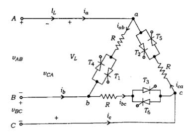
(b) Explain three-phase full-wave deltaconnected controller with various waveforms. a) A single-phase half-wave converter shown in the figure below is operated from a 120 V, 60 Hz supply and the resistive load is  $R = 10 \Omega$ . If the average output voltage is 50% of the maximum possible output voltage, calculate the delay angle, the r.m.s. and average output currents:
