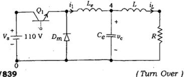
(b) Write on the steady state analysis of buck converter.
