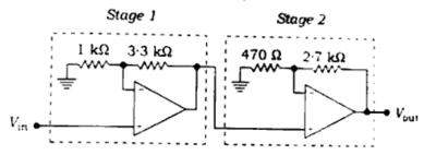
(c) Calculate the voltage gain of this amplifier circuit  $(A_V)$ :
