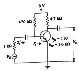
(b) Calculate the value of  $R_1$  in the biasing circuit in the figure given below so that the Q-point is fixed at  $I_C = 8 \text{ mA}$  and  $V_{CE} = 3 \text{ V}$ :
