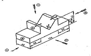
4. The following figures show the top, front and side views of an object. Draw the isometric view of the object: https://www.akubihar.com
