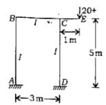
Analyze the rigid jointed frame by moment distribution method. Draw SFD and BMD.
