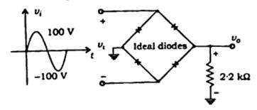
In addition, determine the maximum current through each diode.
