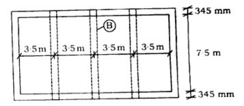
The slab is cast monolithically with beam. The beams are spaced at 3.5 m c/c. The slab is 130 mm thick and design for a superimposed working load of 6 kN/m<sup>2</sup>. The web of the beam is 300 mm wide. Design beam-B using LSM. If M-25 concrete and Fe-500 grade steel is used, design for flexure as well as shear.
