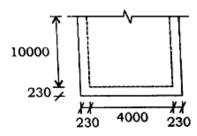
It is subjected to an LL of 4 kN/m<sup>2</sup> and surface finish of 1 kN/m<sup>2</sup>. Consider M-25 concrete and Fe-500 steel.
